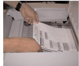
If the ballot is not found in the tray, remove the rear panel by pulling tab sideways and out.
