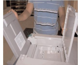
Remove the clean-out tray by pushing in on the flat round tabs at the sides and rolling it forward towards the screen.
